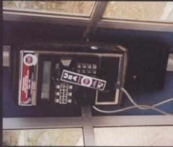
Looking closer, we can see that this is a card-only phone with the coin return and coin box missing, which is why it seems so squat.
